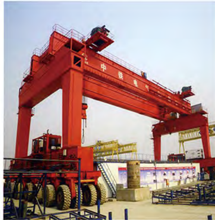
Rubber Tyred Girder Crane
