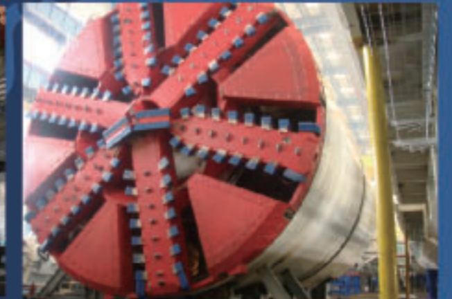
Shield tunneling machine
